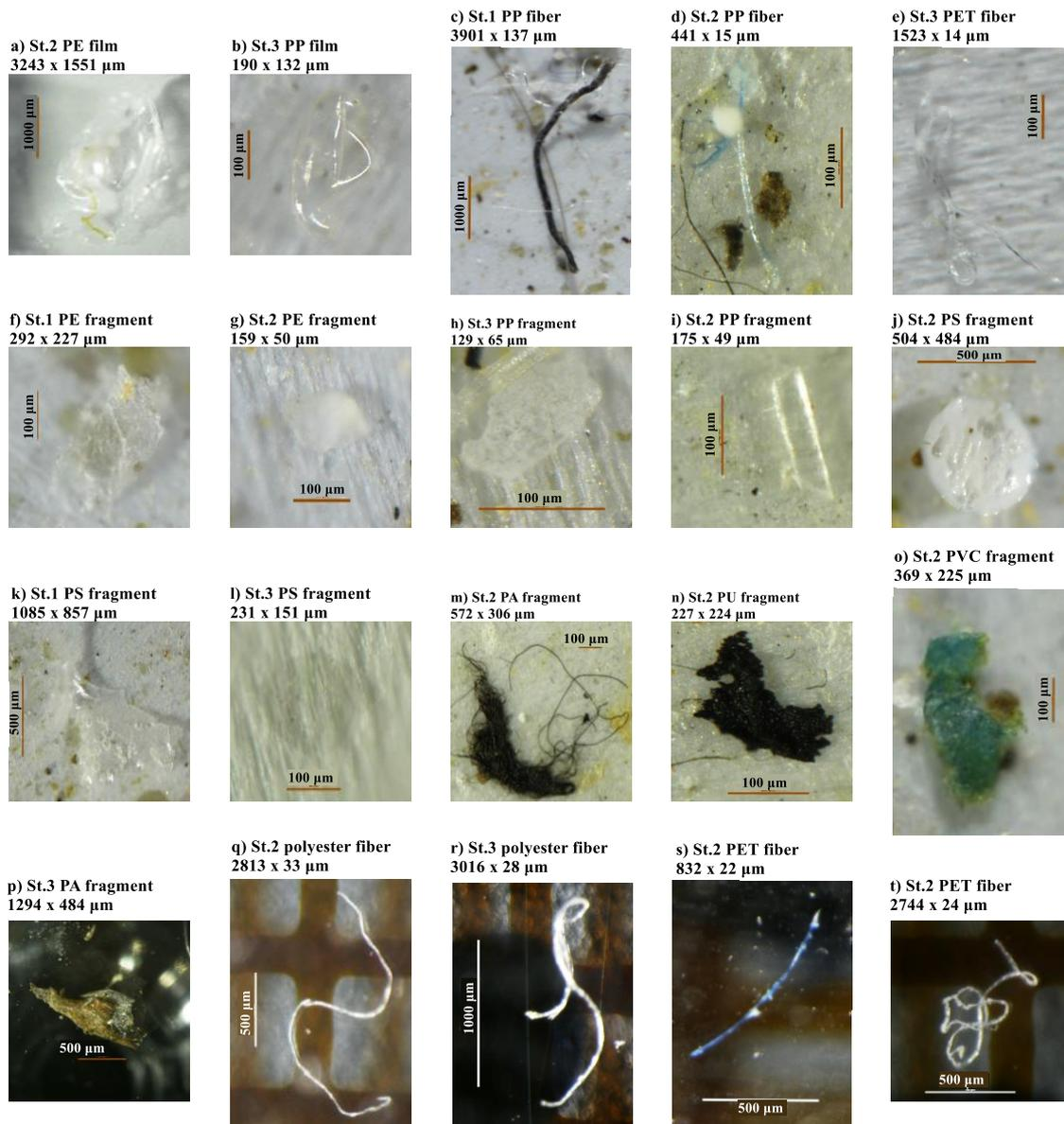
**Figure 18.** The photographed representative microplastics by the Stereoscopic Zoom Microscope (3.0-15.0x) in the 100 (a-o) and 355  $\mu\text{m}$  (p-t) meshes.
