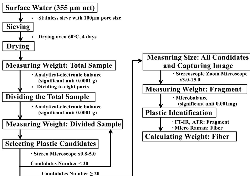
**Figure 10.** Flowchart of laboratory analysis for microplastics collected by the 355 µm net. The Kudo et al. (2018) method was modified and employed.
