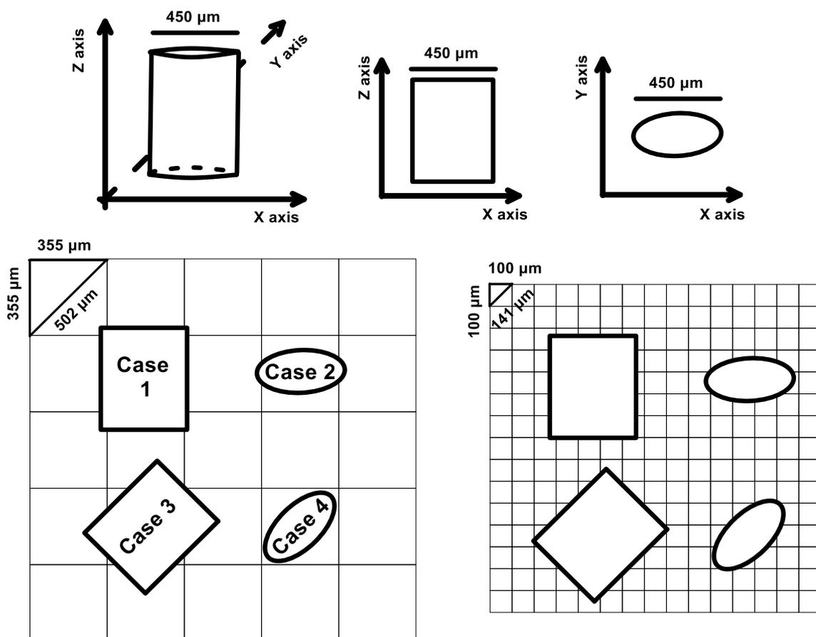
**Figure 15.** The maximum length on the diagonal that appeared in 100 and 355  $\mu\text{m}$  nets. A virtual oval cylinder particle can be collected on the 355  $\mu\text{m}$  net (Case 1-3) and where it is likely to pass through the 355  $\mu\text{m}$  net (Case 4). The figure was extracted from Abeynayaka et al. (2020), supplemented and re-illustrated.
