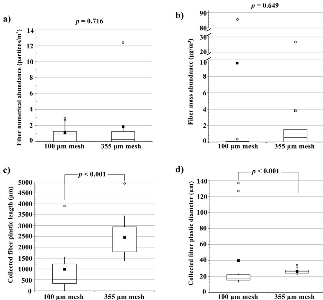
**Figure 19.** Numerical (a) and mass (b) microfibers abundances in 100 and 355  $\mu\text{m}$  meshes and the lengths (c) and diameters (d) of the microfibers.
