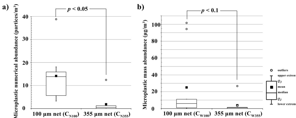
**Figure 13.** The boxplot compared microplastics; a) numerical and b) mass abundances between the 100 ( $C_{N100}$ ,  $C_{W100}$ ) and 355  $\mu\text{m}$  ( $C_{W355}$ ,  $C_{N355}$ ) meshes ( $n=9$ ).
