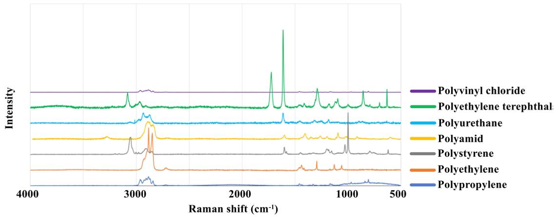
**Figure 11.** The spectra of seven polymer types found in the present study. a) FT-IR and b) Raman spectroscopy. a) The reference spectra in the FT-IR library, b) Commercial product spectra.
