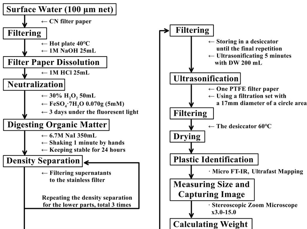
**Figure 9.** Flowchart of laboratory analysis for microplastics collected by the 100 µm net. The Sugiura & Takada (2018) method was modified and employed.
