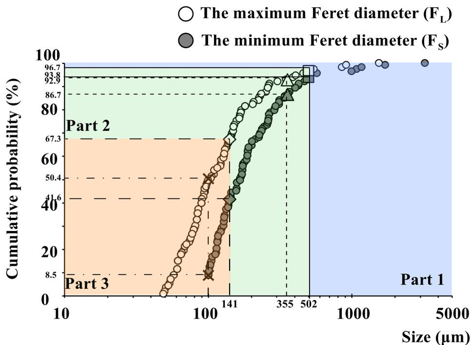
**Figure 16.** The cumulative probability plot of particles (film and fragment) size using the maximum ( $F_L$ ) and minimum ( $F_S$ ) Feret diameter in the 100  $\mu\text{m}$  net. The x-symbols ( $\times$ ) refer to the cumulative probability at 100, the diamonds ( $\diamond$ ) at 141, the triangles ( $\triangle$ ) at 355, and the squares ( $\square$ ) at 502  $\mu\text{m}$ .
