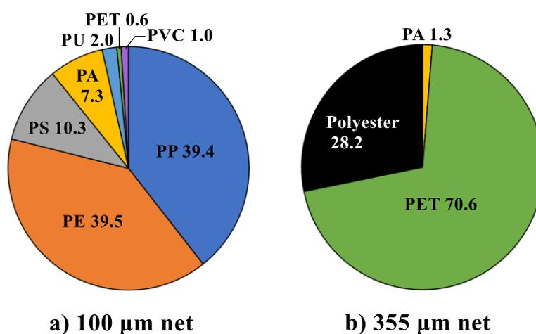
**Figure 20.** Microplastic polymer compositions collected by; a) 100 and b) 355  $\mu\text{m}$  nets.
