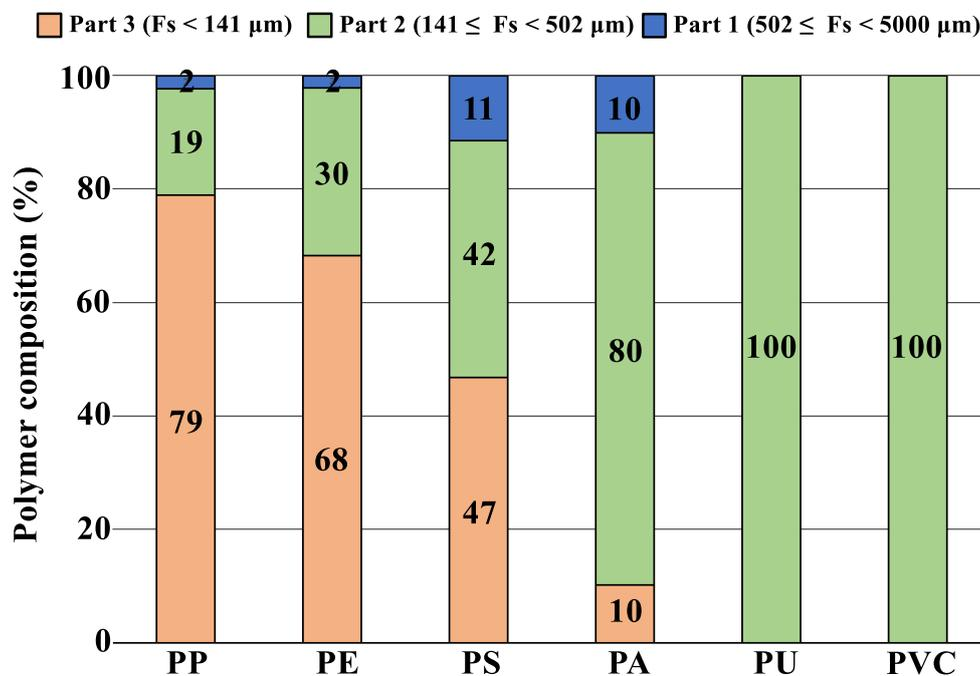
**Figure 21.** Six polymer compositions, which were detected from fragment and shape types in 100  $\mu\text{m}$  mesh, were categorized by three Parts based on the minimum Feret diameter ( $F_s$ ).
