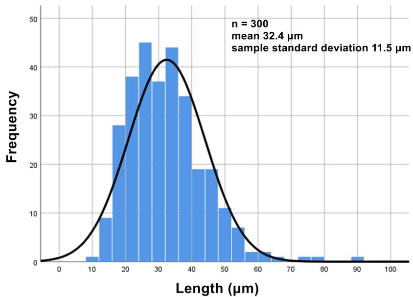
**Figure 32.** The histogram for the sizes of suspended matters in surface water in Nanjung (St.4) 2020, in Citarum River, West Java, Indonesia.
